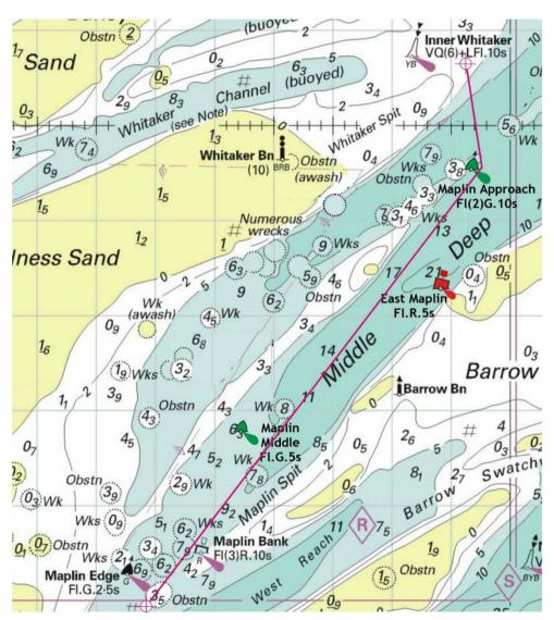
For actual passage via the Middle Deep and benefit from the visual marks following the moves, regard Sector C6 as a direct track from the Maplin Edge waypoint (existing waypoint 23) to the Maplin Approach starboard hand buoy (note the direction of buoyage is towards the Thames) and then a shorter Sector C7 from the Maplin Approach buoy to the Whitaker Spit waypoint (existing waypoint 25).
